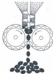
working principle of dry powder briquetting press
